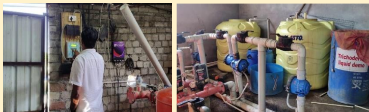
Assembly of automated drip irrigation at Verma's farm, automated scheduling control panel and Venturi system
